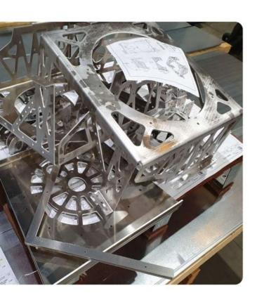
LUMINUM: It is the main material used on the final robot. We use it for plates and folded sheets. It is less sturdy than steel but lighter. We also need help from our sponsors to machine it.
