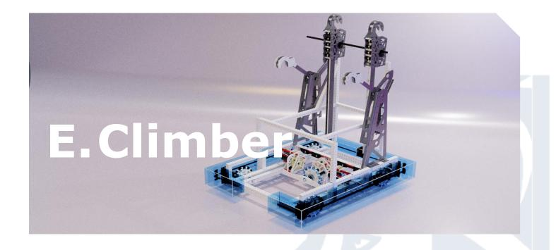
The climber is made of 2 parts: the two climbing arms that pull up and two rotative arms that pivot to tilt the robot towards the next rung once hanging on the HANGAR. Both mechanisms are placed on the back of the robot to use its center of mass to help the robot climb. The climber is designed to directly reach the second rung and is powered by the drivetrain's PTO.
