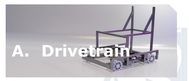
During the off season, we imagined an OMNI drivetrain. It consists of setting four OMNI wheels on the frame and one in the center of the drivetrain, but in reverse direction. The main advantage is the handling: with this type of drivetrain, we could move laterally. When our drivetrain was conceived, our driver was still unsure with which type of drivetrain he would be more comfortable. That's why we thought of a way to convert our OMNI drivetrain to a tank one by shifting the wheels' position.
