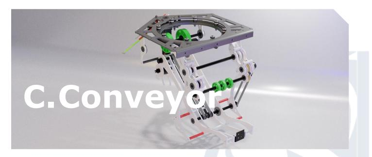
On our former robot, the conveyor was untrusted, and balls got stuck inside the mechanism. We tried to build a more reliable prototype. This new mechanism is positioned horizontally to widen the space and stock up to two CARGOS.
