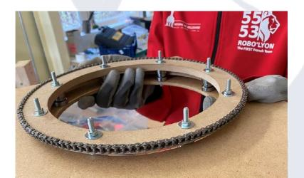
For this mechanism, we were inspired by the design of a tank turret. So, we prototyped several iterations in order to have the smoothest rotation and the most accurate turret possible.
