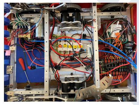
For electronics parts: We designed a custom-made electronical plaque using our CNC, allowing us to manage our cable easily.
