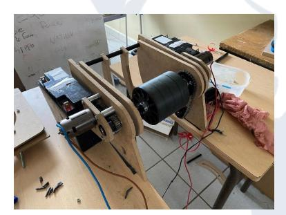
To shoot power cells, we almost immediately came up with the idea of a shooter consisting of a single set of wheels in order to be more accurate by giving the ball a Top spin effect, causing a straighter trajectory and giving the shooter a better precision. With this kind of shooter, we can also choose the exit angle of the ball, enabling us to reach our power port from almost anywhere on the field.
