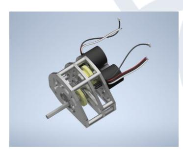
At first, we designed a two speed ballshifter gearbox in order to have one speed dedicated to torque and the other one to velocity. But as our robot was way too heavy for the game, we redesigned a much lighter version to fit the rules.
