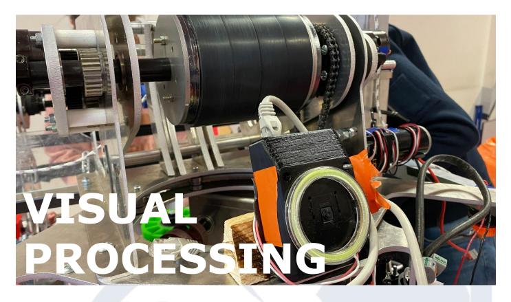
This year, we focused our efforts on the visual processing, as it is particularly important in Infinite Recharge. We've decided not to use the Limelight camera, so we instead use a Raspberry Pi with the chameleon visual processing program which allows us to know our relative angle with the power port. The image is provided by a PiCamera surrounded by a green LED Circle.
