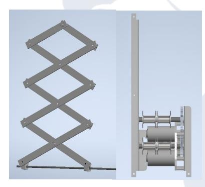
To climb on the generator switch, we've envisaged two radically different mechanisms. The first in the form of a scissor lift. Although this design was the most practical, it was pretty big so we would have lost precious space for the other mechanisms. The other idea was a telescopic arm paired with a winch. This solution enables us to gain space as the winch isn't mounted on the floor of the robot but rather on reinforcement higher on the drivetrain.
