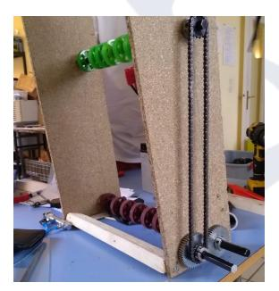
We BUILT a prototype of a mechanism which could catch balls. We used ANDYMARK green and maroon compliant wheels, motorized by a CIM motor. It allowed us to test the spacing between the wheels and to check if this kind of mechanism was working to catch and expel the balls.
